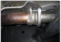
INSTALL HEADPIPE # A INTO STOCK PIPE. USING BOLT KIT PROVIDED INSERT WELDED HANGERS INTO RUBBER GROMMET.. DO NOT TIGHTEN.
